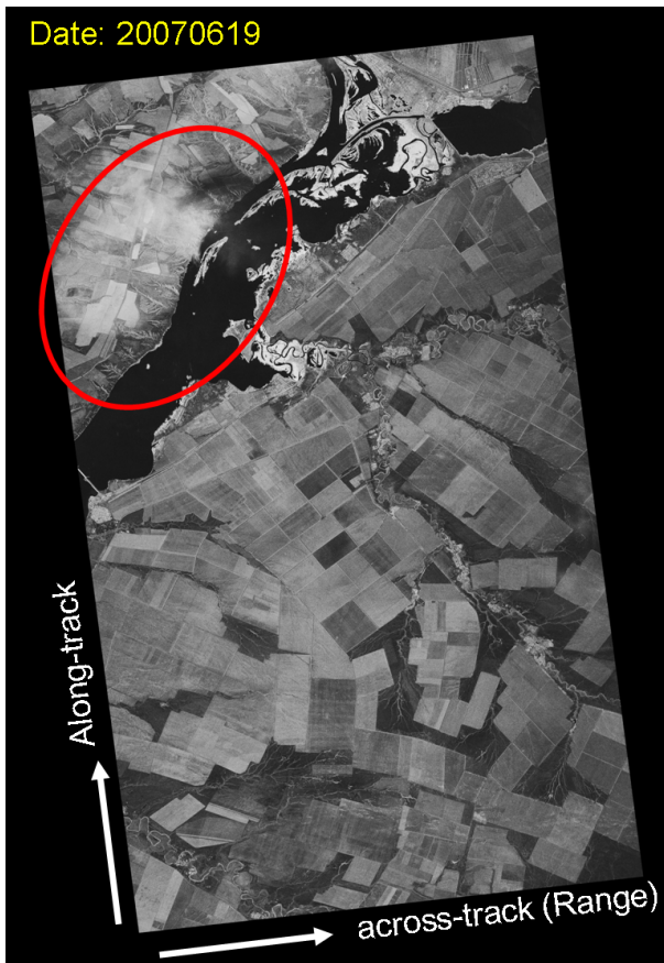
Fig. 1. An example of rain-cell-affected SAR signatures recorded with TerraSAR-X. The white shading is due to direct reflections from the rain region (shown as volume 'A' in Fig. 2). Whereas the darkly shaded areas are due to rain attenuated (blocked) signals from the ground; this effect is shown as region 'B' in Fig. 2. The parameters of acquisition are given in Table I.
