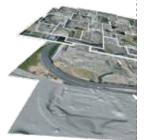
With its 16MP high resolution camera, the **eBee** can capture images with a ground resolution of 3 to 30cm per pixel. Areas from 1.5 to 10km<sup>2</sup> can be mapped in a single flight depending on image resolution and flight altitude.
